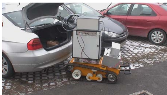
Figure 6 GUARDED robot platform approaching a suspicious box in a car trunk (top) and an alarm for chloropicrin is set off on the laptop computer connected to the platform via WiFi (bottom).
