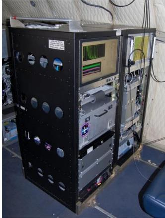
The IONICON PTR-TOFMS installed aboard the NASA research aircraft. (Picture: NASA)
