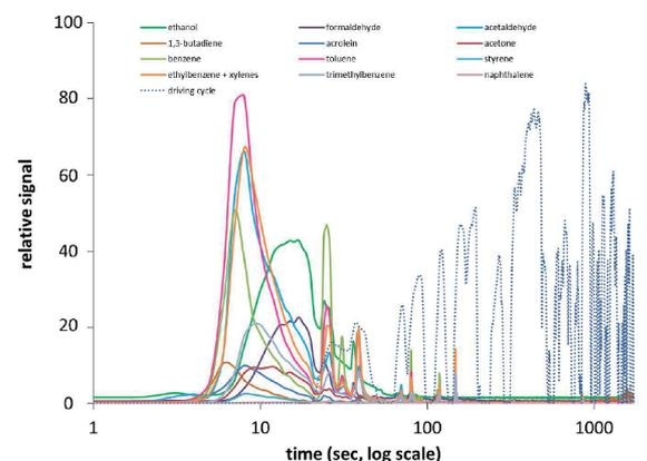
Fig. 3: Emissions from gasoline vehicle exhaust.
