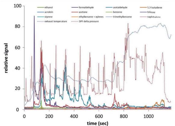
Fig. 2: Emissions from diesel vehicle exhaust.
