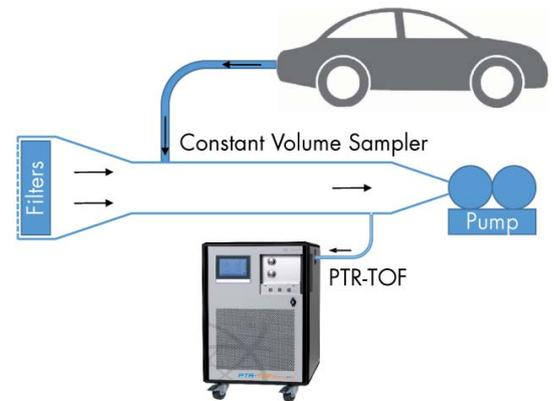
Fig. 1: Typical setup for real-time automotive exhaust monitoring with an IONICON PTR-TOFMS instrument. It includes a dilution system, such as a constant volume sampler and a heated sampling line to minimize surface interaction of semi volatile compounds.
