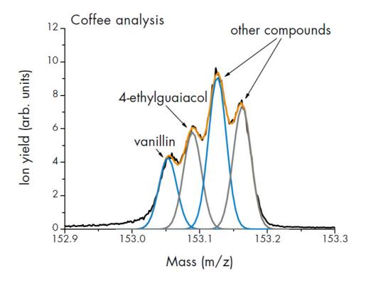
The four different isobaric ions, which can be clearly separated and quantified independently with high resolution PTR-TOFMS, would appear as a single signal at nominal m/z 153 in a SIFT-MS instrument. This means that, for example, hazardous substances cannot be separated from harmless compounds and protonated molecules cannot be distinguished from fragments in SIFT-MS if they are isobars.
