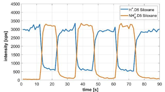
Figure: Fast switching between proton transfer ( $\text{H}_3\text{O}^+$ ) and adduct ionization ( $\text{NH}_4^+$ ) in ~1s. This includes switching between high and low reaction energies (E/N).
